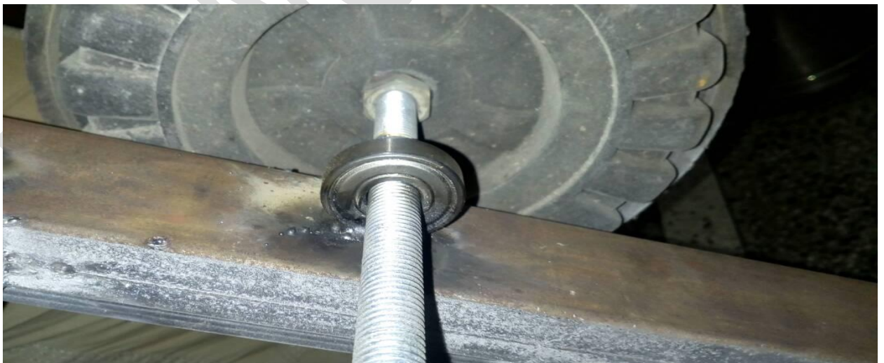
Fig. 5.4 Bearings are Welded on the Frame
