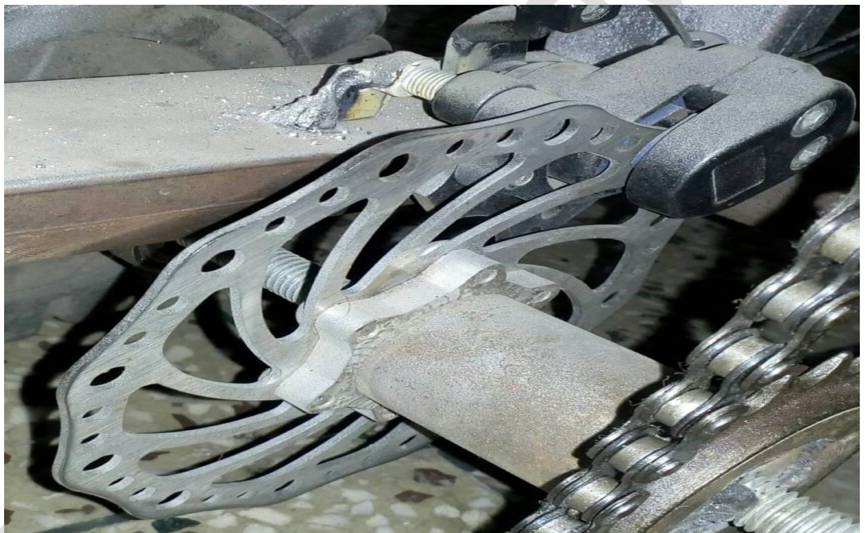
Fig. 5.5 Disc Brake Connected with Rear Axle
