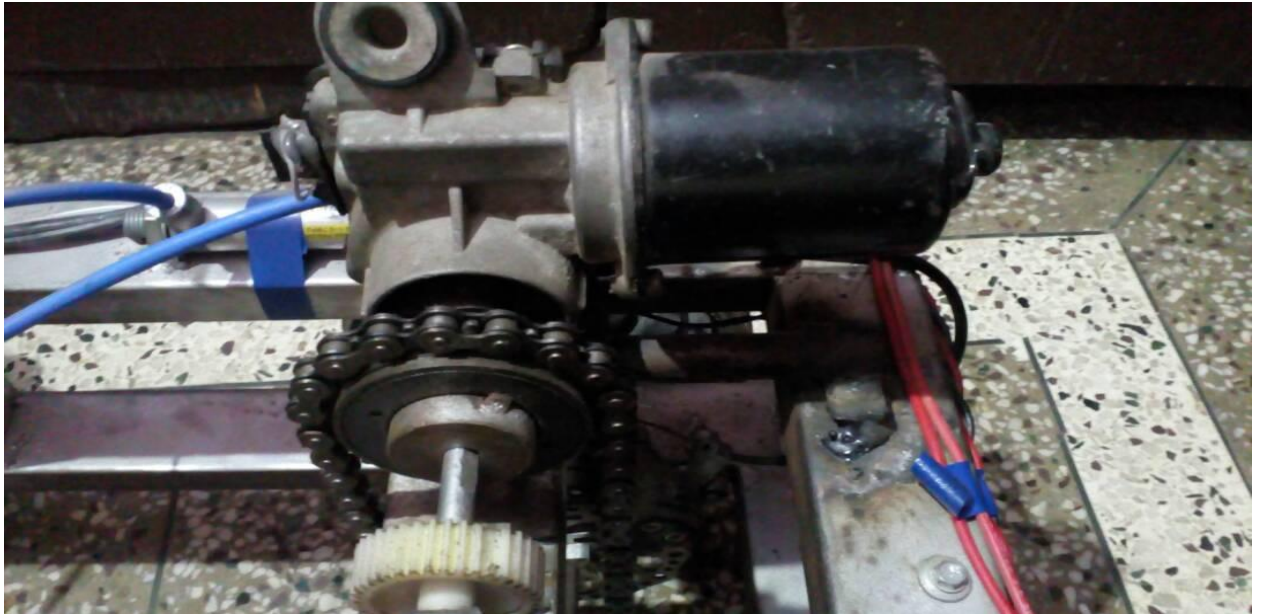
Fig. 5.6 DC Motor Attached with Sprocket
