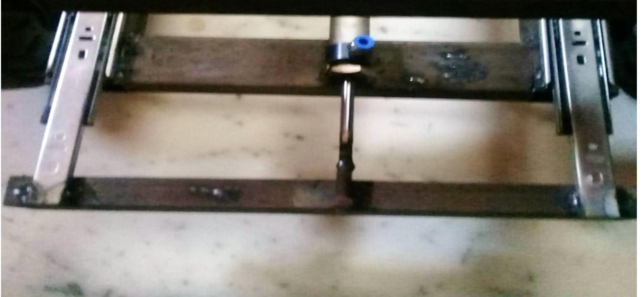
Fig .5.1 Bumper is Welded with Sliding Channels
