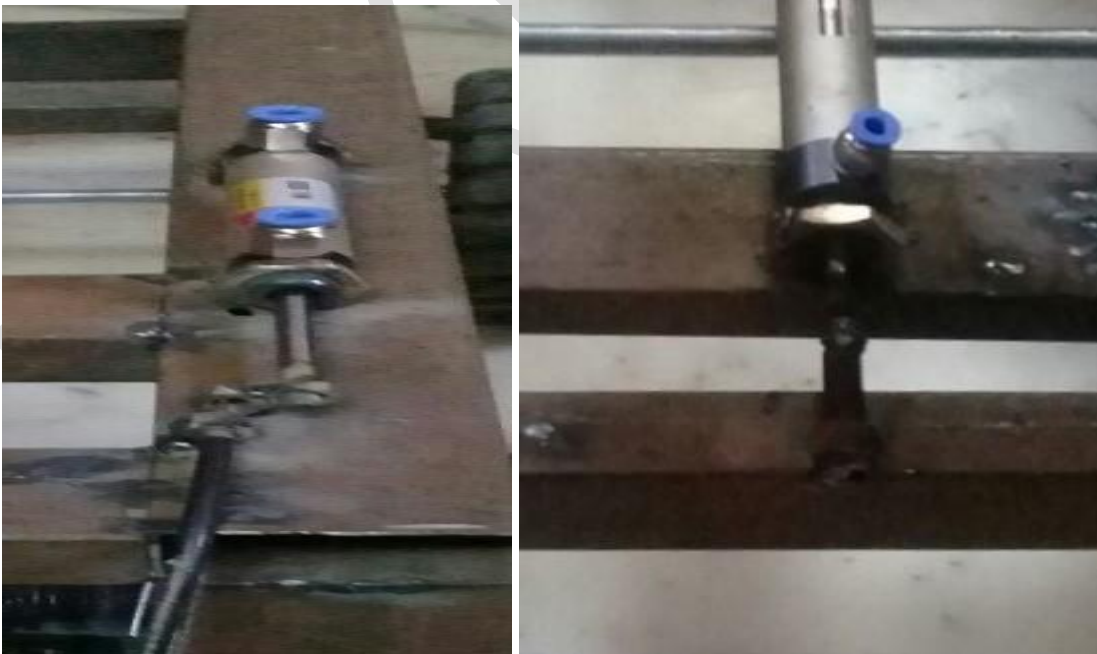
Fig. 5.2 Brake Connected with Cylinder
