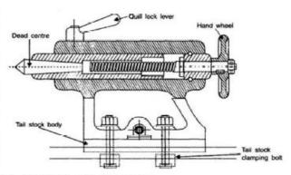
lever or lock handle is used to hold the tailstock spindle in a fixed position.
