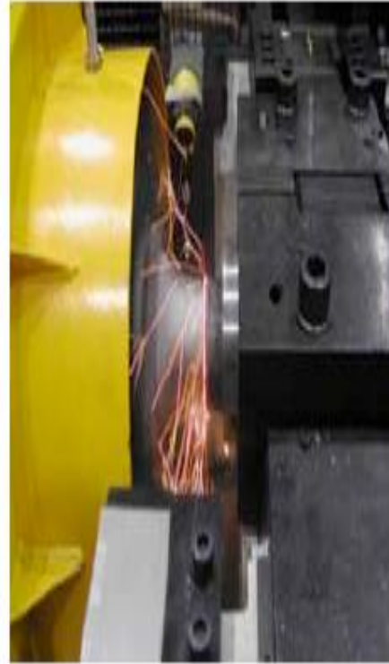
(b) First friction The chuck is accelerated to speed and parts brought in to contact.
