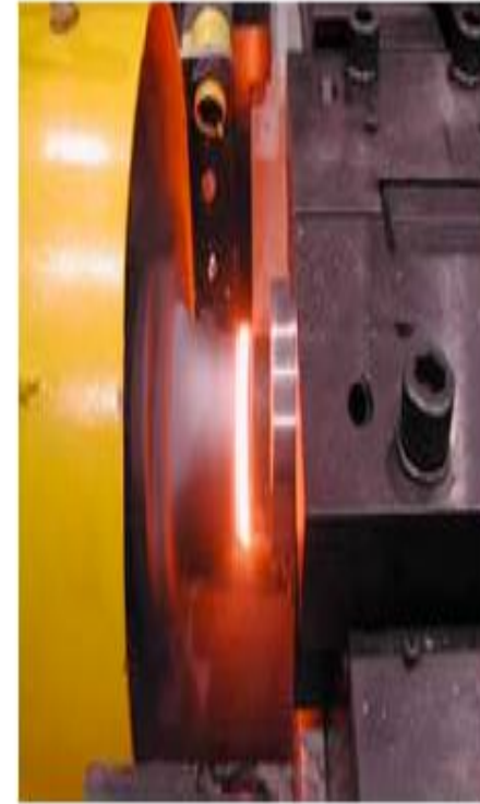
(c) Second friction The force is plastic material starts To extrude from the weld interface.
