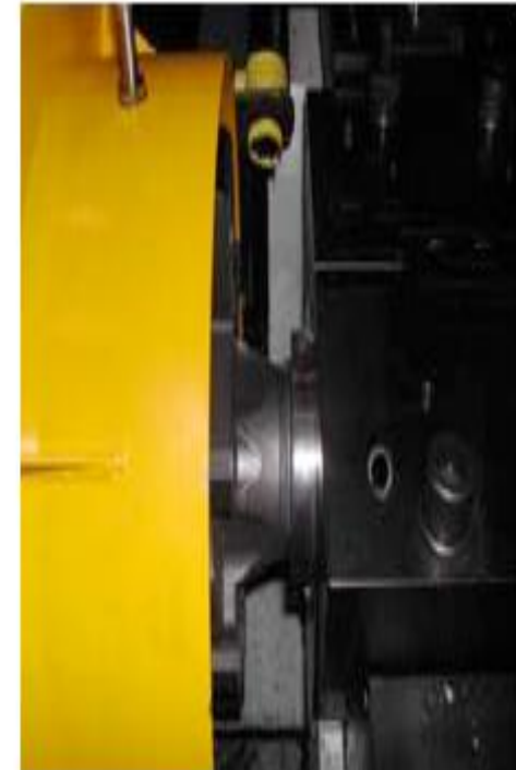
(f) Weld complete The weld is complete a full area, homogenous Bond.
