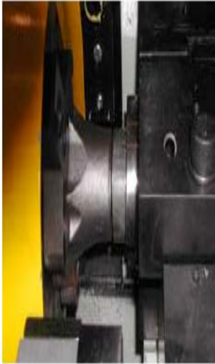
(a) Pre friction One part is held stationary In a fixed clamp. The other Part is held in a rotating Chuck.
