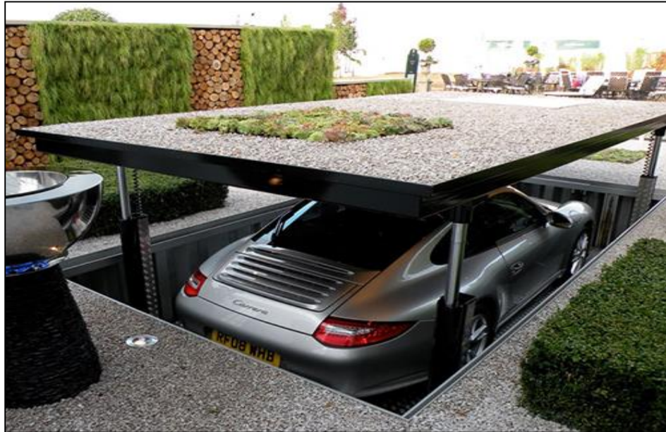
Fig. 1.6 Underground Hydraulic Car Parking System
