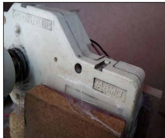
Fig. 5.11 Gearbox with DC Motor
