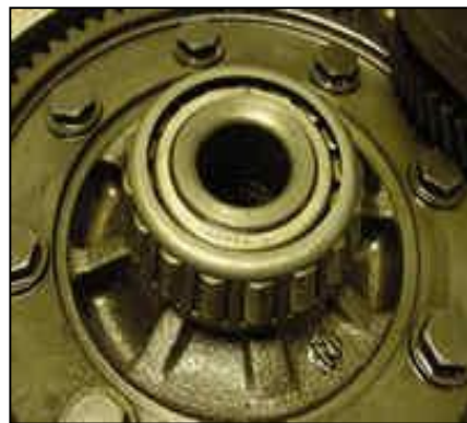
Fig. 3.5 Tapered Roller Bearing from a Manual Transmission [5]
