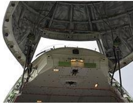
Fig. 17 – Leadscrews are used to raise and lower the front door of the Boeing 747-8F Freighter aircraft.
