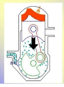
Transfer/Exhaust: Towards the end of the stroke, the piston exposes the intake port, the allowing compressed fuel/air mixture in crankcase to escape around the piston into the main cylinder. This expels the exhaust gasses out exhaust port, usually located on the opposite side of the cylinder. Unfortunately, some of the fresh fuel mixture is usually expelled as well.
