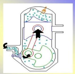
During the downward stroke the poppet valve is forced closed by the increased crankcase pressure. The fuel mixture is then compressed in the crankcase during the remainder of the stroke.
