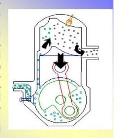
Compression: The piston then rises, driven by flywheel momentum, and compresses the fuel mixture.
